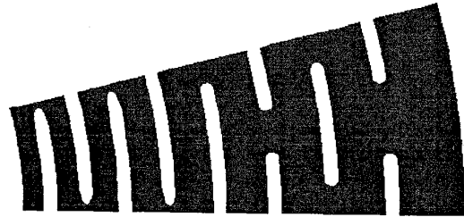
Fig. 3d Staggered elongated cooling hole design with semi-elliptical ends.
